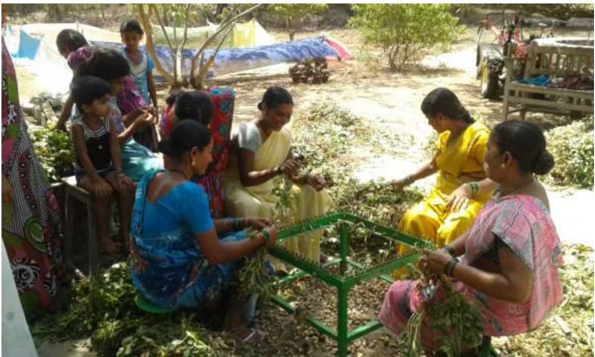
Fig 2 : Practical session on groundnut stripping with the help of women friendly groundnut stripper
