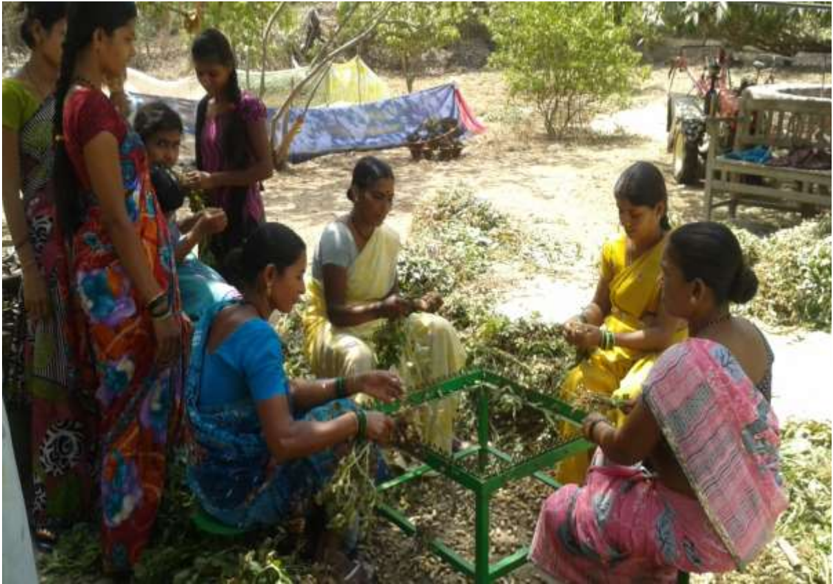
Fig 1: Practical session on groundnut stripping with the help of women friendly groundnut stripper
